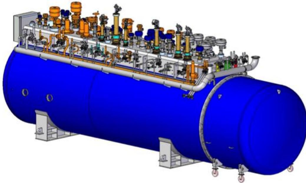
One Coldbox comprising 6 expansion turbines, 3 cold compressors, built-in acceptance test equipment
